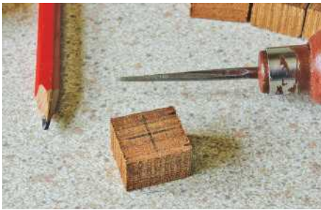
▲ Pic.10 Mark the centre of the block for centre popping; Bernard uses a carpenter's finger gauge
